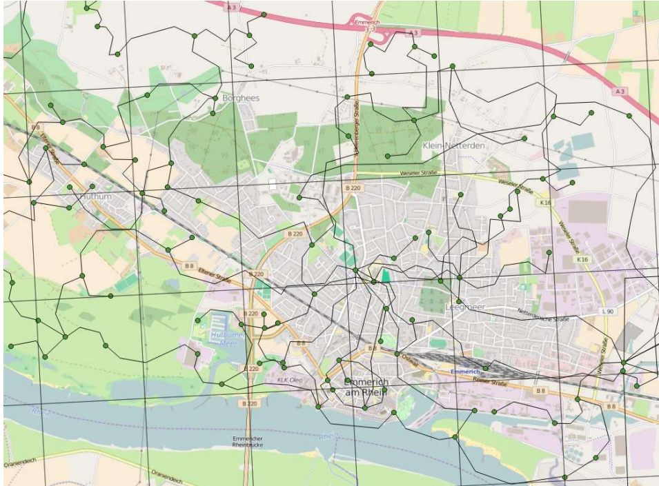
Figure 45 Area of Emmerich with German 1km*1km grid and power nodes and lines (map: OpenStreetMap)
