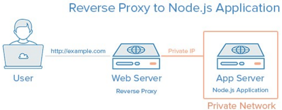
Figure 16: Server-user communication workflow with NGINX reverse proxy [NODE].
