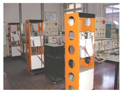
Figure: Practical setup of Herakles platform with 3 power electronic converters, interconnected via a TCP/IP based info'structure.
